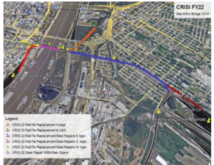
MacArthur Bridge aerial showing improvement projects
