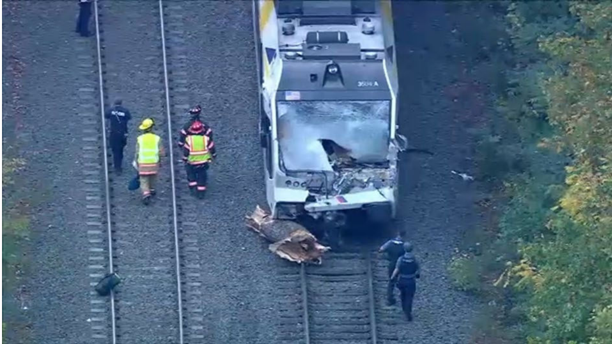
Figure 1. Aerial view of damaged train and portion of struck tree in their final positions. (Source: 6abc Action News.)
