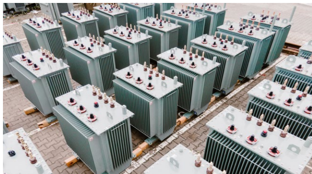
Recycled mineral oil-filled transformer
