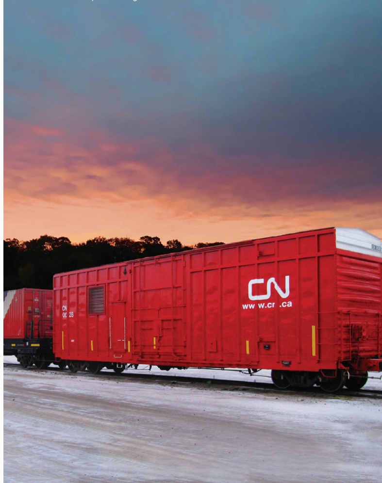
CN's distributed air braking cars supplement the air supply to a train's air brake system during colder weather.
