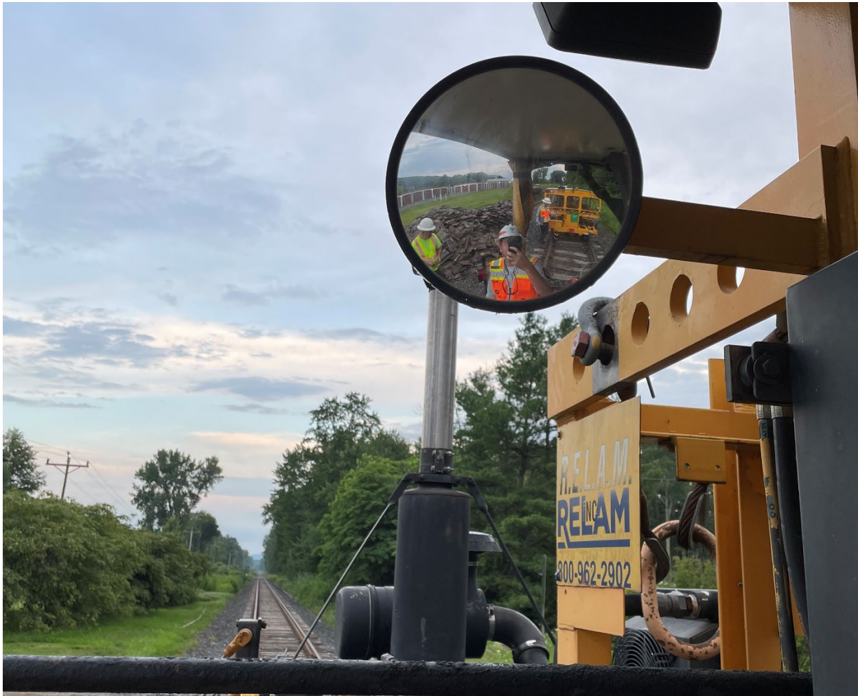
Figure 7. The field of view in the driller’s rearview wide-angle mirror from the driller operator’s seat. (Courtesy of the FRA.)
