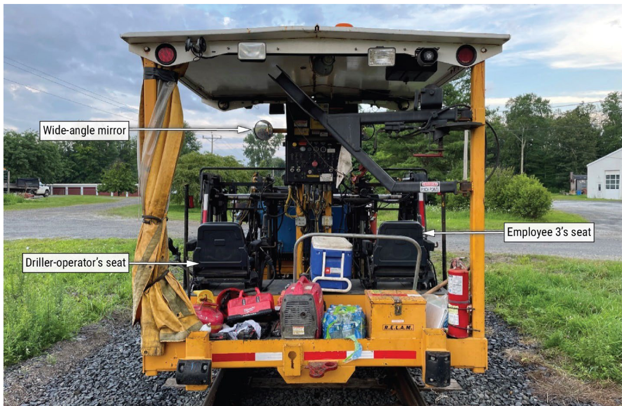
Figure 6. Rear view of the tie driller RMM. (Courtesy of the FRA).
