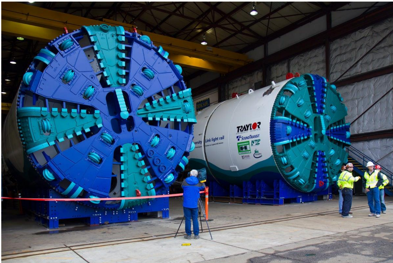
Figure 2-1 Twin Bore Transit TBMs
