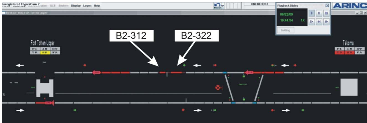
Figure 7. Example of Advanced Information Management controller display showing status of signals, interlockings, track circuit occupancies, and train movements between Fort Totten and Takoma stations. Contiguous solid red blocks indicate presence of a train. (Icons for track circuits B2-312 and B2-322 indicate that these track circuits are reporting as occupied without a train present.)
