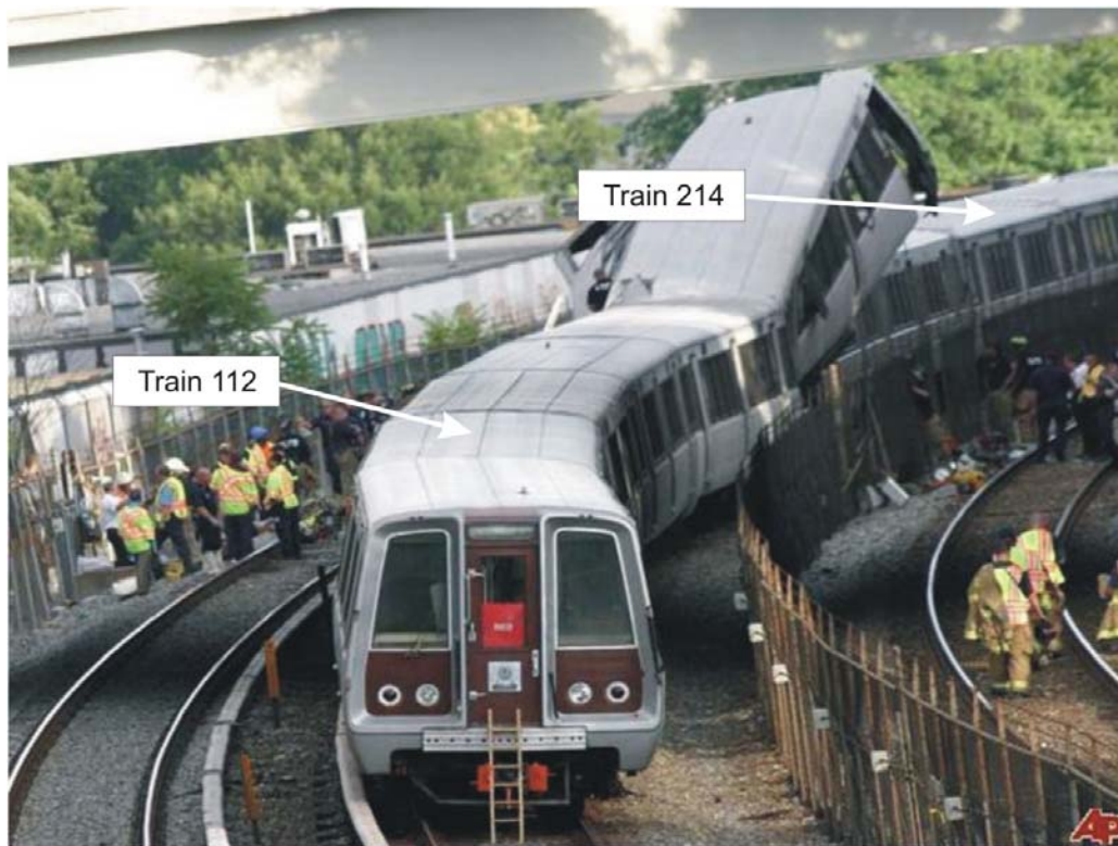
Figure 1. Lead car of striking train (train 112) has overridden last car of struck train (train 214), which has telescoped into lead car of train 112.
