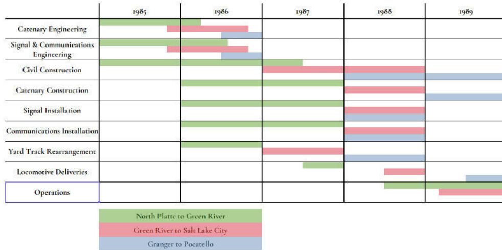
Figure 4. Planned Construction Timeline for the UP Electrification
