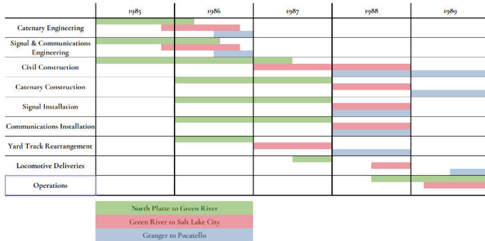
Figure 4. Planned Construction Timeline for the UP Electrification
