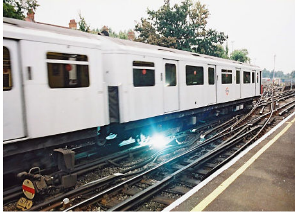
Figure 17. Visible Arcing Between the Lead Rail Vehicle’s Shoe and One of the Energized Rails on the London Underground (SPSmiler, 2005)
