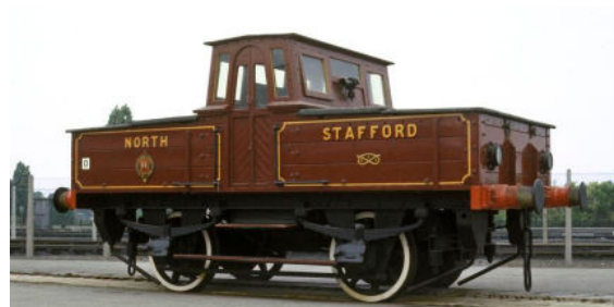
Figure 10: Battery locomotive from 1917 in the United Kingdom 54
