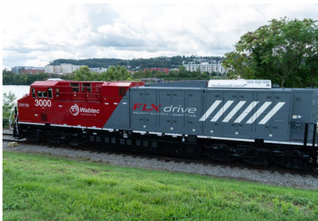
Figure 11: Wabtec 2.4 MWh FLXDrive battery locomotive 58
