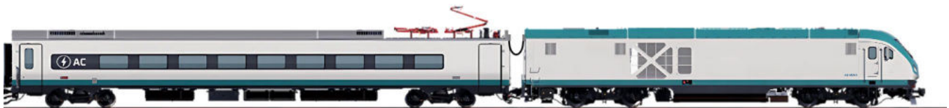
Figure 17: Diesel-electric locomotive with AC catenary power on the passenger car
