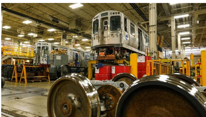
Quarter-life overhaul work being performed on CTA's 5000-Series railcars.
