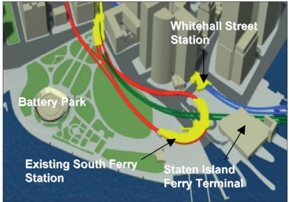
The 98-year-old South Ferry Station is built on a curve as a single-loop track (pictured above), which slows operations. Planning is under way for a straight, two-track terminal that will allow all 10 cars to platform (instead of just five) and help reduce transit times for Staten Island commuters and Statue of Liberty and Ellis Island visitors.
