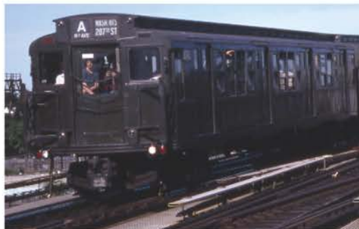
The R1-R9 series (R9 pictured) were built between 1930 and 1940. They were the first cars procured by the IND. The R stands for "Revenue Contract," a designation still used today.
