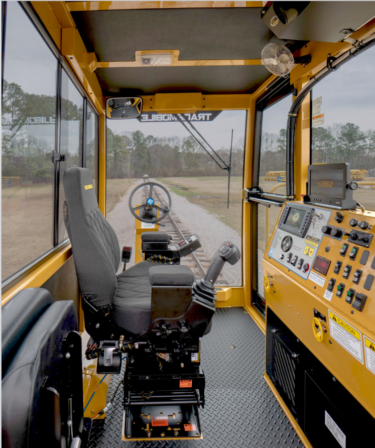
Atlas control panel and operational controls.
